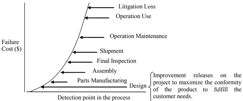
Figure 1 – Failure costs versus failure detection point [2]
