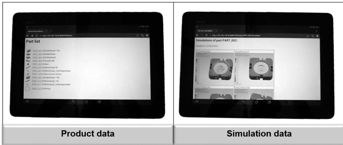
Figure 15: Example view of the retrieval of a part list (a) and simulation results (b) using a web browser on a tablet computer
